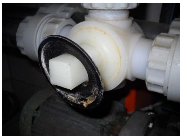
Figure 2: Examples of identified contamination sources of Lactobacillus parabuchneri in milking systems. A contaminated tube of the end unit of a milking system with milk deposits (picture left) and a contaminated three-way valve of a pipe milking system (picture right) (Maurer et al. 2016).
