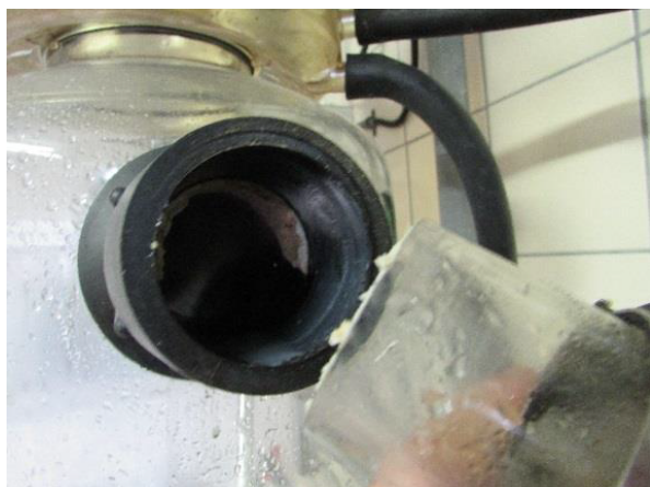
Figure 2: Examples of identified contamination sources of Lactobacillus parabuchneri in milking systems. A contaminated tube of the end unit of a milking system with milk deposits (picture left) and a contaminated three-way valve of a pipe milking system (picture right) (Maurer et al. 2016).
