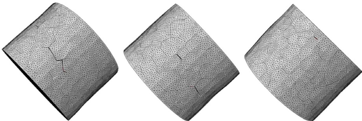
**Figure 1.** Cracks in an assembly of 700 grains (meshed by 1,000,000 elements) at 20% strain.
